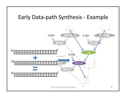
Hence, we can replace the 16-bit addition by a 8-bit addition and a bit-concatenation.
