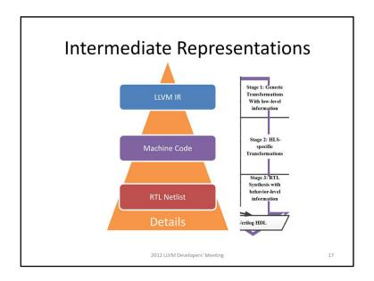
The closer to the end of the low the IR located, the more details are exposed.
