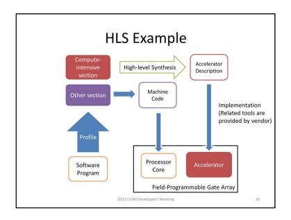
So given a program to run on these device, we can first profile the program to identify the "compute-intensive section" and then implement it as hardware accelerator, with the help of a HLS tool.
