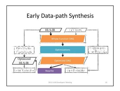
We call the bit-level/subword-level optimiations and Technology mapping in the cross-level engine as "Early Data-path Synthesis". I will give an example of the "Early Data-path Synthesis" on the machine code before scheduling and binding. Essentially, it builds an whole function DAG, perform optimize on it and rewrite it back.
