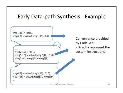
Because the HLS-specific operations are directly expressed by the MachineInstructions. We can directly analysis the rewritten Machine code to get the delay/cost estimation.
