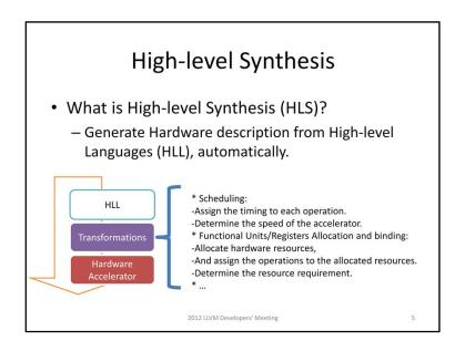
During the transformation process, there are two key tasks should be perform: That is Scheduling and Resource allocation and binding.
