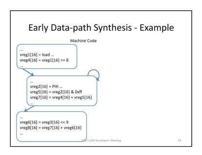
Supposed we started from this piece of machine code. It contains addition, bit-wise and and shift. As well as load and PHIs
