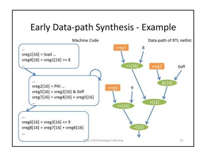
First of all, a DAG is built according to the Machine Code.
