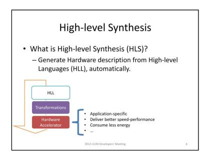
At last HLS generate the description for the hardware accelerator, which describe the structure and the timing of the circuit. With the Hardware accelerator, we can achieve better speed-performance while consuming less energy, at the cost of hardware resource usage and development time, comparing to implementing the same functionality with general-propose processors.
