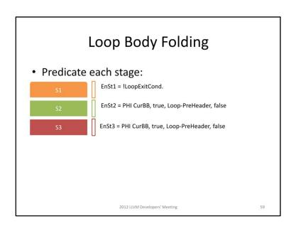
To fill and flush the pipeline correctly, we also need to predicate each stage.
