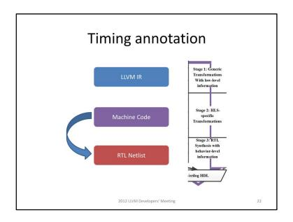
The timing information will also be annotated to the RTL Netlist, which means retiming with scheduling result is possible.
