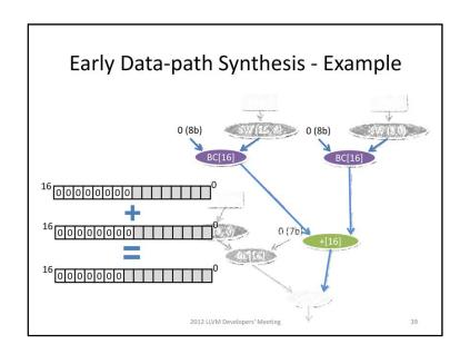
At the same time, bit-concatenation can provides the bit-mask information explicitly. Hence we could take the advantage of the bit-mask to optimize the arithmetic operations.
