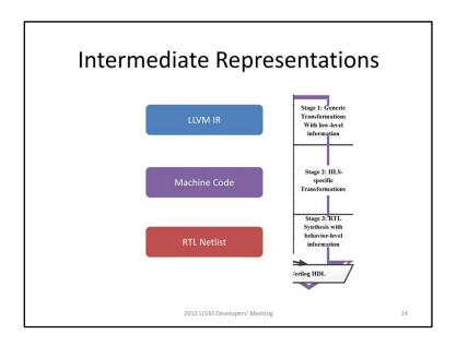
There is different kinds of IRs for each stages in the synthesis flow, including LLVM IR, Machine Code and RTL Netlist.
