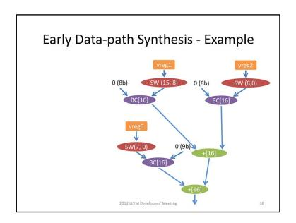
By applying similar optimizations, we can obtain a netlist like this, we replaced nodes by subword-extraction and bit-concatenation whenever possible, because these two operations are zero cost in the hardware accelerator.
