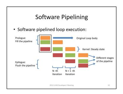
Software pipelining is a type of out-of-order execution, except that the reordering is done by a compiler.
