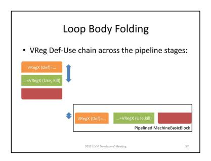
After loop-body folding the Def-use chains are also folded, this may result in a wrong live-interval and even break the SSA-form.
