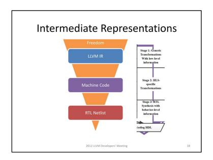
But the freedom of transformations is also reduced at the low level, because they need to preserve the constraints inherit from the High-level IRs.
