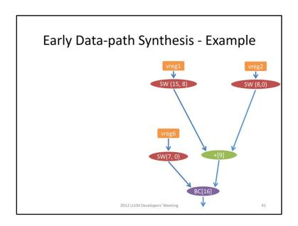
Finally we can get a netlike this, you can see that the operations are replaced by the ones that have a lower cost.
