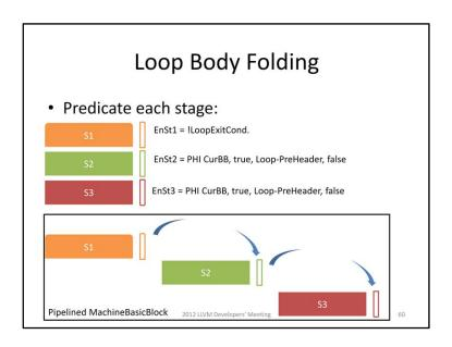
By constructing the predicate chain carefully, we can propagate the stage enable correctly.
