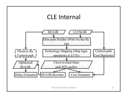
Specifically, it first build a close-to-final data-path netlist with bit-level/subword-level optimiations and Technology mapping. With the close-to-final netlist, we can either rewrite it back to high-level IR, or estimate its implementation cost.
